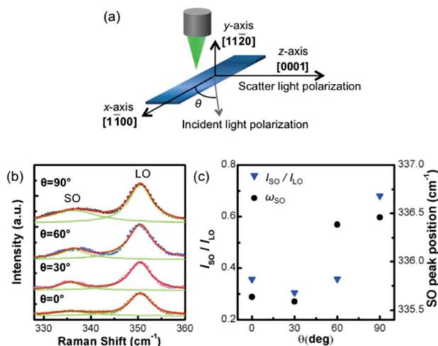
**Fig. 4** (a) Schematic illustration of the polarization dependent Raman measurement. (b) Polarization dependent Raman spectra measured from a single ZnS NB with different angles. (c) Angular dependency of  $I_{\text{LO}}/I_{\text{SO}}$  and  $\omega_{\text{SO}}$ . Single ZnS NB with different angles. (c) Angular dependency of  $I_{\text{LO}}/I_{\text{SO}}$  and  $\omega_{\text{SO}}$ .
