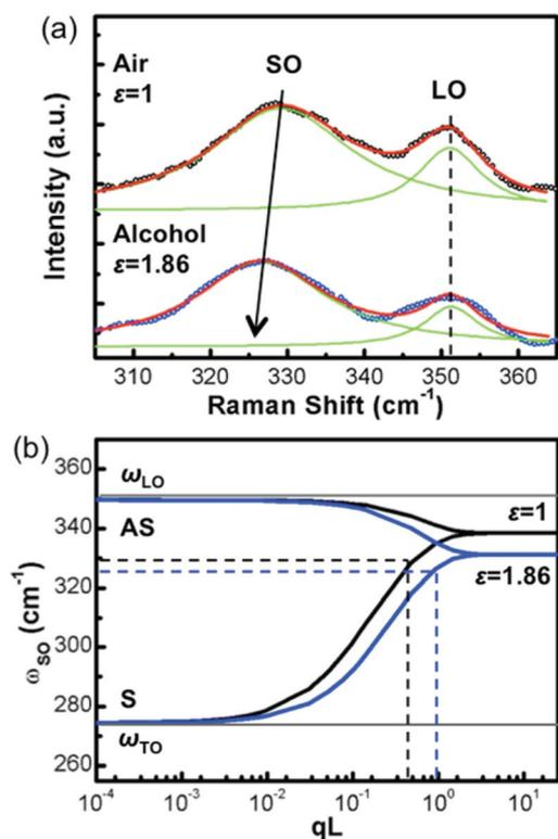
**Fig. 3** (a) Raman spectra measured in the surrounding material with different dielectric constants (air and alcohol); (b) calculated SO phonon dispersion relation in air and alcohol.  $q_i L_i$  is (the phonon wavevector)  $\times$  (the feature size of the ZnS NBs).
