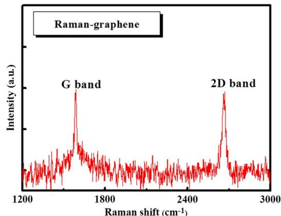
**Fig. 2.** Raman spectrum of pristine graphene using 633-nm He-Ne laser.
