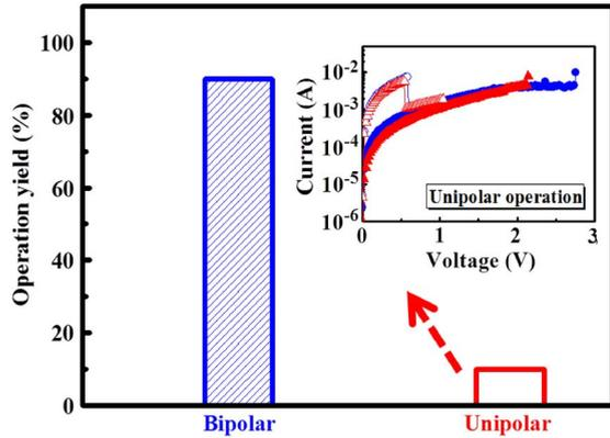
**Fig. 4.** Probabilities of switching modes of the ZnO memory with graphene electrodes, including both unipolar and bipolar operations. The devices are chosen randomly to conduct the statistics.
