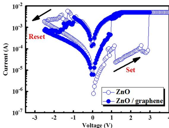
**Fig. 3.** Typical resistive switching behaviors of the ZnO TRRAM device with and without graphene electrodes. The positive bias induces the LRS and the negative bias resets the HRS.
