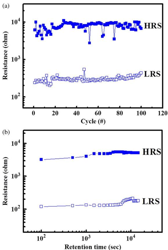
**Fig. 6.** (a) The evolution of resistance states of and graphene/ZnO device during the 100 resistive switching cycles. (b) The nonvolatile property of both HRS and LRS of graphene/ZnO devices at room temperature.
