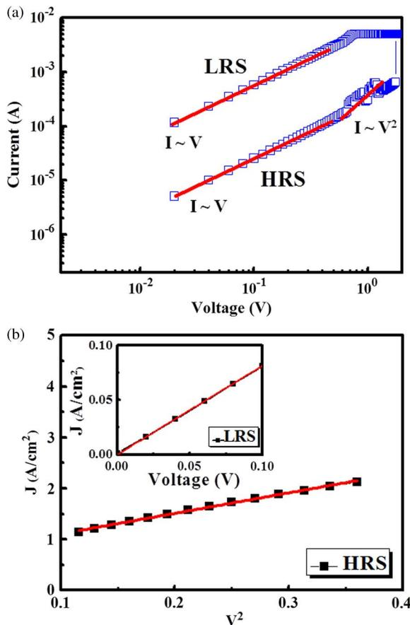
**Fig. 7.** (a) Conduction properties of the graphene/ZnO device. (b) Linear fitting of LRS and HRS in the graphene/ZnO device.
