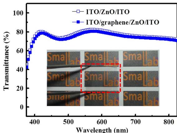
**Fig. 1.** The transmittance of ITO/ZnO/ITO/glass (open squares) and ITO/graphene/ZnO/ITO/glass (solid squares) devices within the visible region from 400 to 800 nm. The inset shows the fabricated ITO/graphene/ZnO/ITO TRRAM device. The background can be observed through the device without any refraction or distortion.
