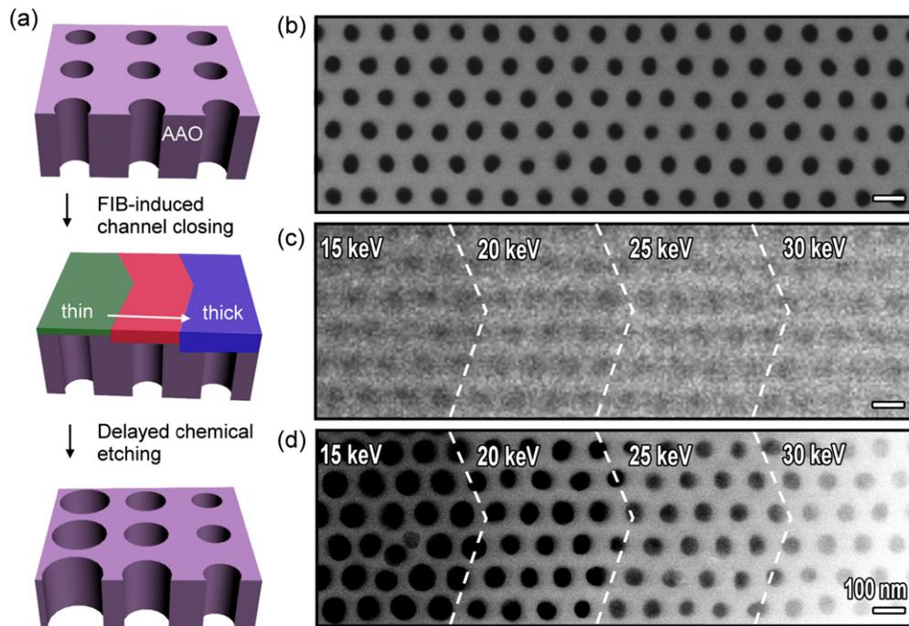
**Figure 4.** (a) Schematics showing the fabrication process to create the AAO template with nanochannels of different pore sizes. (b) and (c) SEM images of an ordered array of AAO nanochannels before and after being covered by capping layers created by FIB of different energies. (d) Nanochannel arrays with graded pore sizes created after etching (scale bars are 100 nm).
