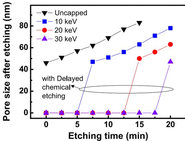
**Figure 3.** Pore size as a function of etching time for nanochannels covered by capping layers created by FIB of different energies.
