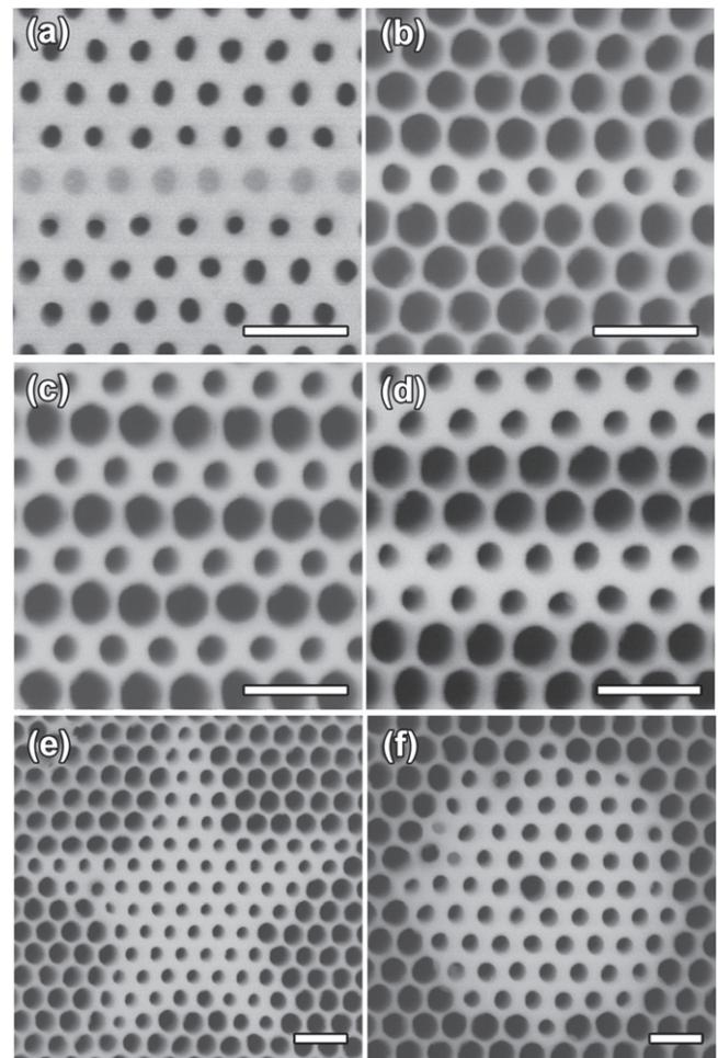
**Figure 2.** SEM images of (a) closed nanochannels arranged in a single line, and nanochannels with two different pore sizes arranged in (b) a single line, (c) single line arrays, (d) double line arrays, (e) star, and (f) a hexagonal array with a nanochannel of larger pore size at its center (scale bars are 200 nm).
